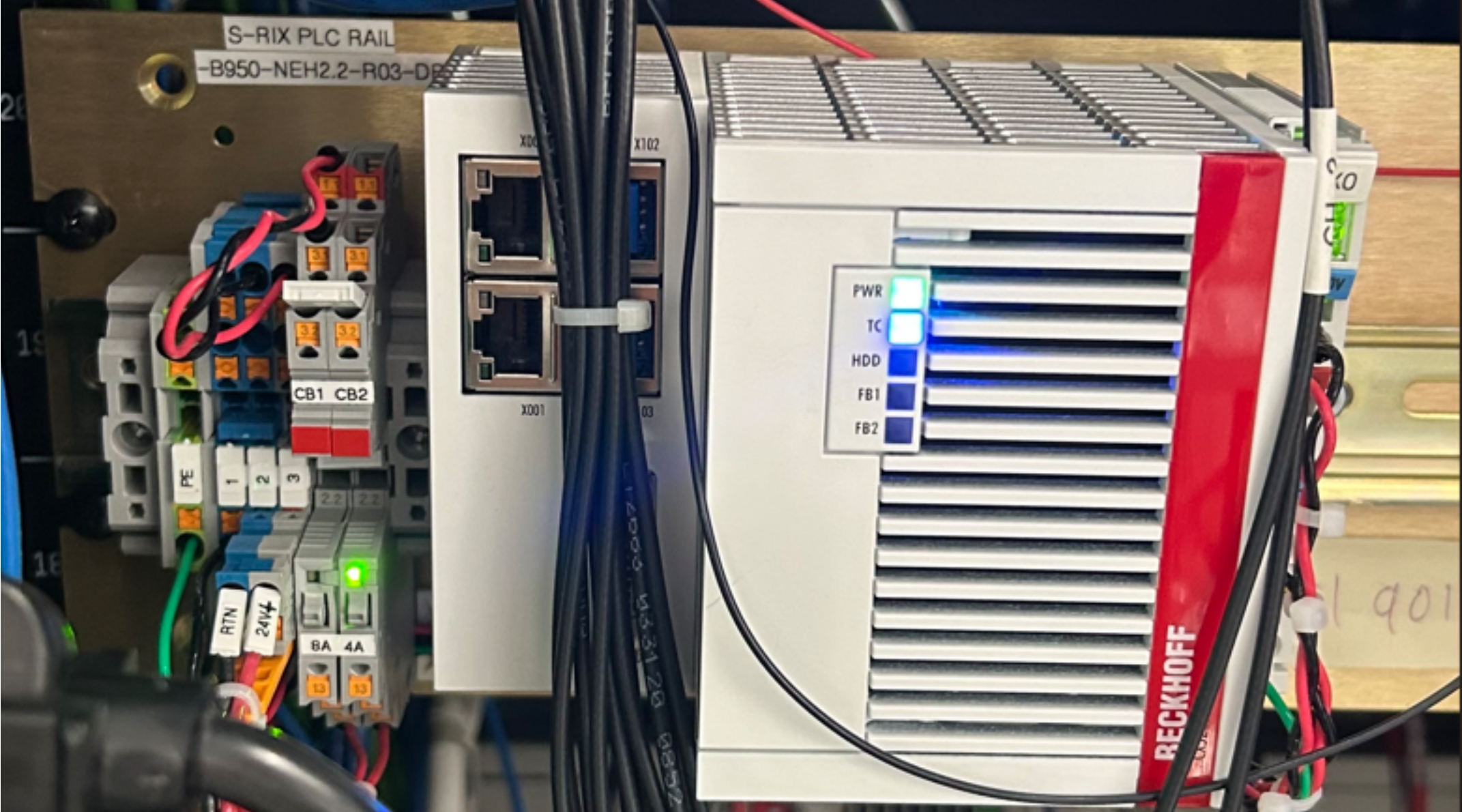
Figure 7. TwinCAT PLC hardware used in the sRIX environment.
