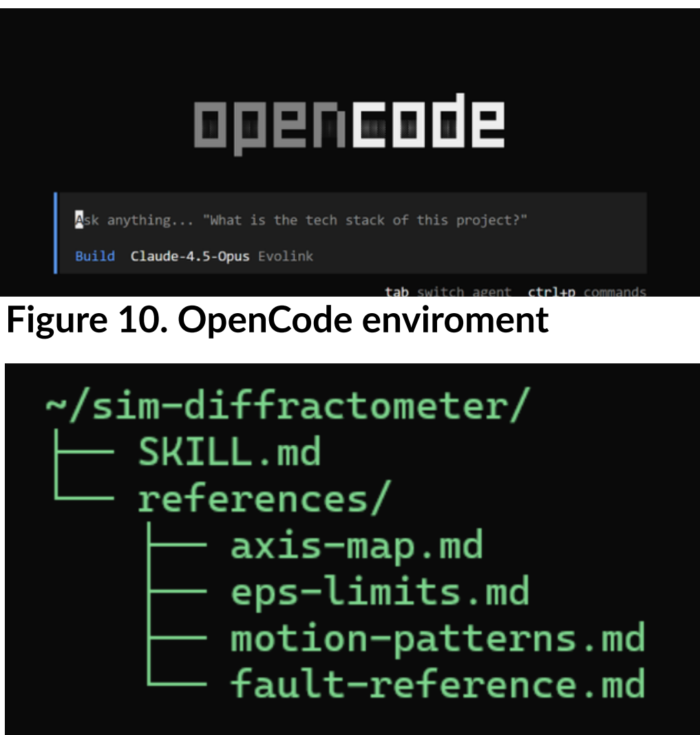
Figure 10. OpenCode environment Figure 11. The copilot agent uses a skill-based design in which a central SKILL.md file defines how the agent should respond to diffractometer. The reference files include axis mappings, motion patterns, safety limits, and elog workflow context. This gives the agent content to reference when reasoning about motor movement.
