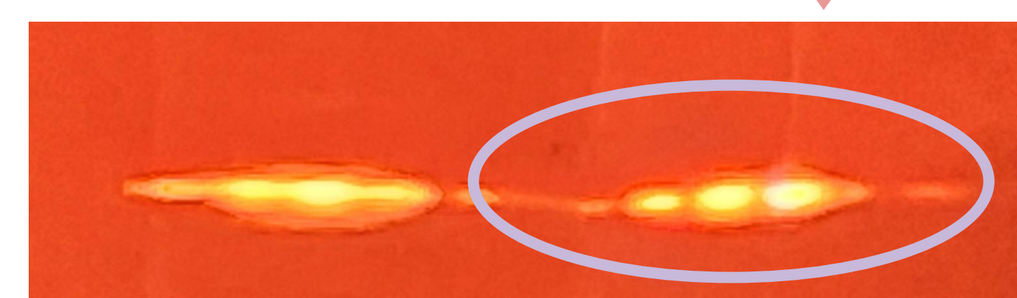
Spectrally dispersed shaped laser pulse viewed on a card just before the 2 nd curved mirror in AOM pulse shaper setup
